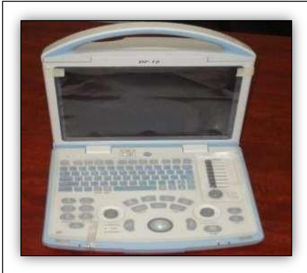
Figure (1): 2D ultrasound device (Mindray Dp 10) with 10 MHZ linear transducer probe
