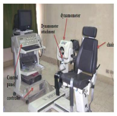
Fig.(1): Biodex system 3 Isokinetic dynamometer.
